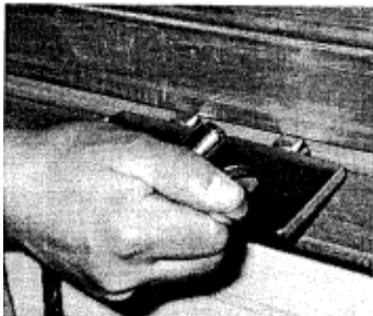
Open Hinge-O'-Grab to 180°, Insert posts into slot in beam
