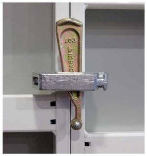
The MEVA clamp is one piece that can be put into place using only one hand. It establishes a secure 5-point connection with a few hammer blows.
