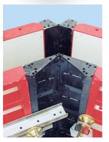
Imperial panels come with a full range of corner options to meet the needs of any project. 90° inside and outside corners are used for standard corner forming. Articulated corners (left) are adjustable between 60° and 180° with a locking device for repeated angles. Stripping corners for stair and elevator core forming (above) collapse into a smaller angle for stripping and movement without disassembly. There are also special corner options for forming columns (right).
